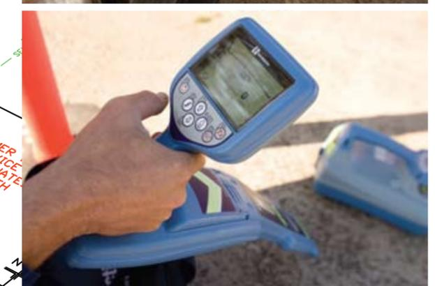
Underground Services Detection was engaged by head contractor Probuild to perform an underground services investigation for the entire site at 401 St Kilda Road, prior to the start of construction. The process started immediately after demolition of the building and infrastructure that previously occupied the site.
