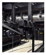
"The additional functionality requirements make the design quite complex, requiring two independently braked 11kW motors and mounting the platform to six SERAPID LinkLifts to lift."
