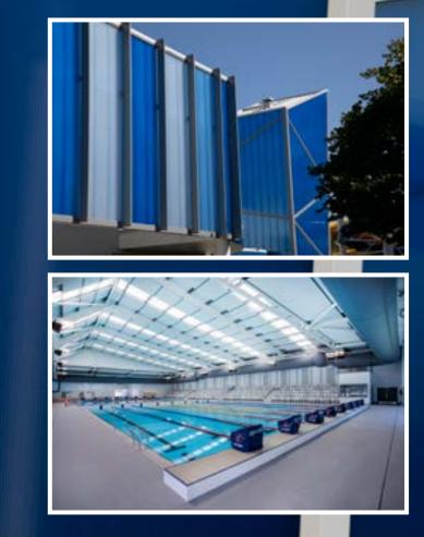
Close Commercial Services are a Melbourne based specialist roofing subcontractor. For the Gippsland Regional Aquatic Centre, they supplied and installed Kingspan roof, Kingspan wall, EEFAS skylight systems, polycarbonate cladding and flashings to make the roof and façade meet airtight requirements.
