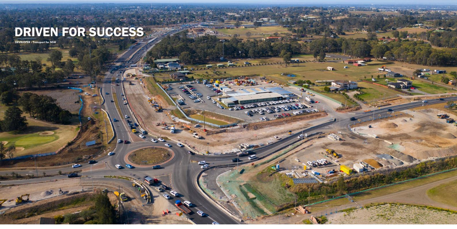
The Northern Road Upgrade Stage 3 is between Glenmore Parkway, Glenmore Park and Jamison Road, South Penrith. Work includes widening the road to provide additional lanes, as well as new traffic light intersections to improve traffic flow and reduce congestion. A new interchange with the M4 Motorway is also being provided as part of the upgrade. The project also includes a new roundabout and service road and upgraded foot paths, drainage, noise barriers, retaining walls, and landscaping.
