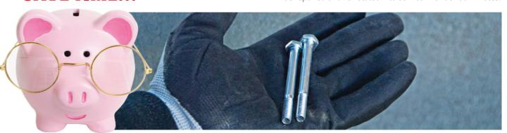
In 90% of all impacts in Australia, the only spare structural parts needed for repairs are 2 shear pins (COST <\$5). After 59 impacts in Australia, the average cost for each reset was \$169.
